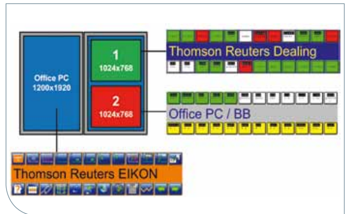
With Focus technology, the programmable soft keys on the WEY keyboard are automatically switched to the functions of the active application
