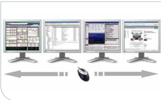
WEY Mouse Switch Solution allows users to switch and toggle between PCs merely by moving the mouse cursor from one screen to another
